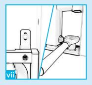
Place the frame back between the joists, and using a socket wrench or spanner secure to the wall and floor using the supplied screws.
