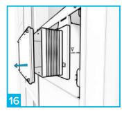
Remove the cover cap prior to completing the wall.
