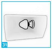
Place the blanking caps onto the ends of the bolts.
