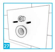
Locate the wall protector membrane and hang against the wall.
