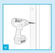
Drill 5mm pilot holes at each marked location.
