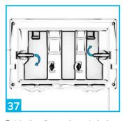
Rotate the clips as shown to lock and secure.
