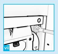
Tighten using a socket wrench or spanner.
