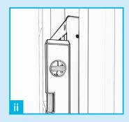
With the feet set flush with the front edge of the joists, ensure the frame is plumb.
