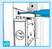
To ensure the frame is plumb, adjust the level of the frame using the adjustment bolts.
