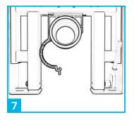
Tighten the height adjustment bolts on both frame legs and check that the height hasn't slipped.
