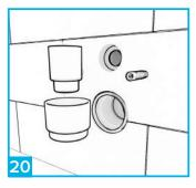
Remove the flush pipe and drain connector blanks.
